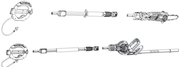
3. To unlock and remove the handle from the telescopic pole, depress the PUSH buttons on both sides of the handle and pull out the handle.
