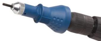
4. Attach the blind riveting attachment as a bit into the drill chuck of the drilling tool. According to the size of the blind rivet nut adjust the torque of the drilling tool. Always start with the lowest torque.
