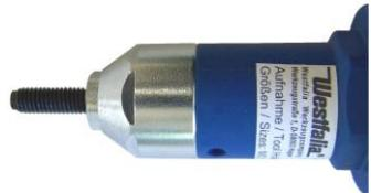
3. Use the included wrench (6) in order to tighten the nosepiece (5) on the head (3) of the blind riveting attachment.
