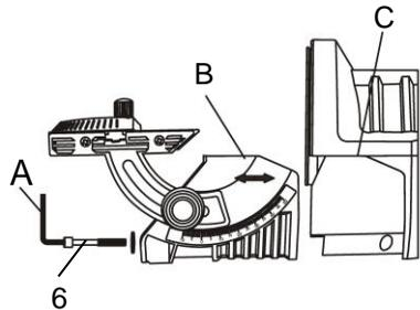
4. To reinstall the sanding table assembly, place it against the bottom of the motor housing (C) and slide it toward the sanding plate. **Note:** Make sure the positioning tabs are fully inserted into the matching slots in the motor housing.
